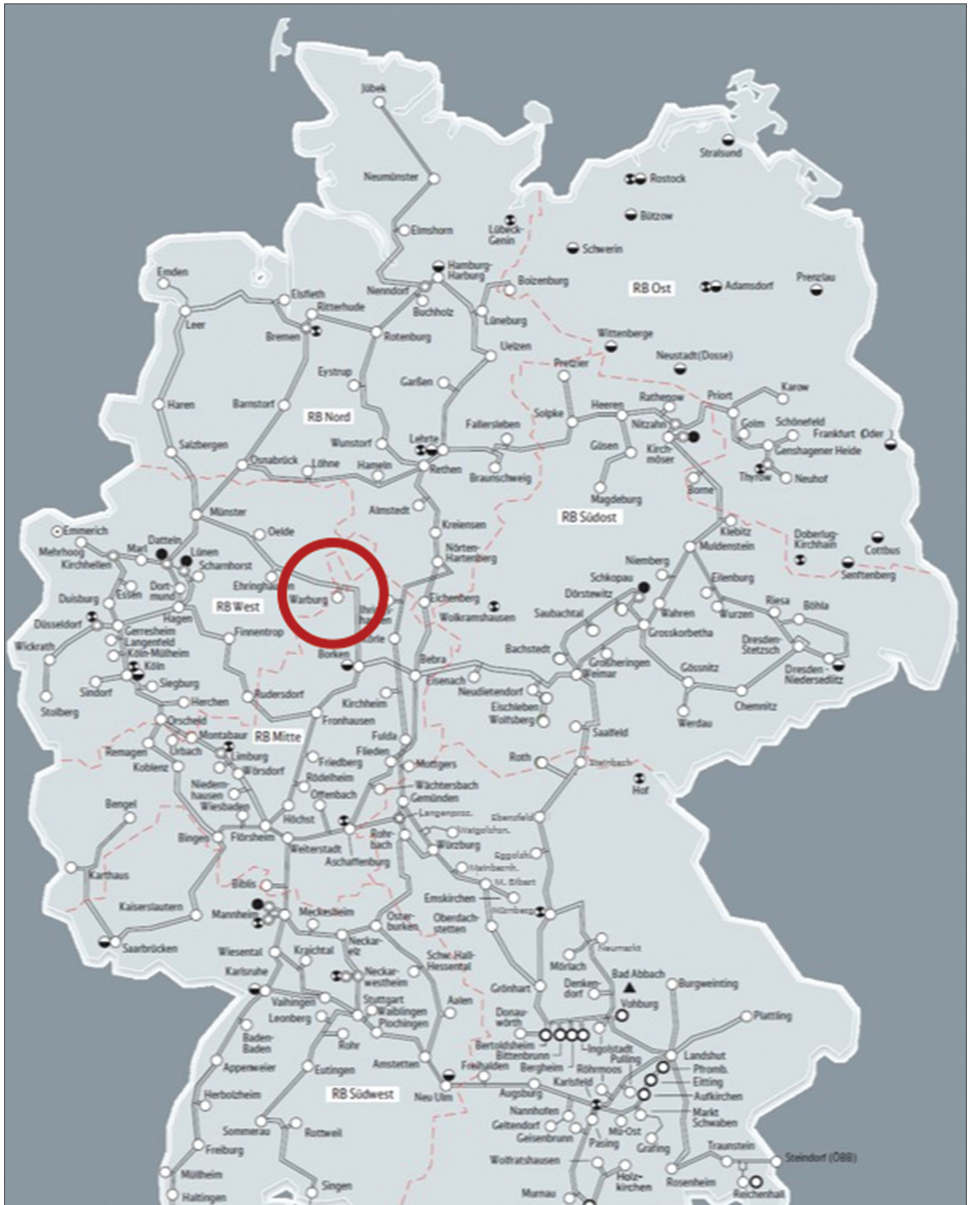
Figure 2: German 110 kV railway traction network with the reference location in Warburg (Source: DB AG)
